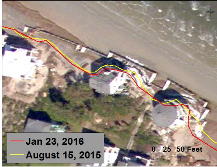
Map 2: Shows the landward movement of the scarp line position at Harbor Island after the WDS was installed.
